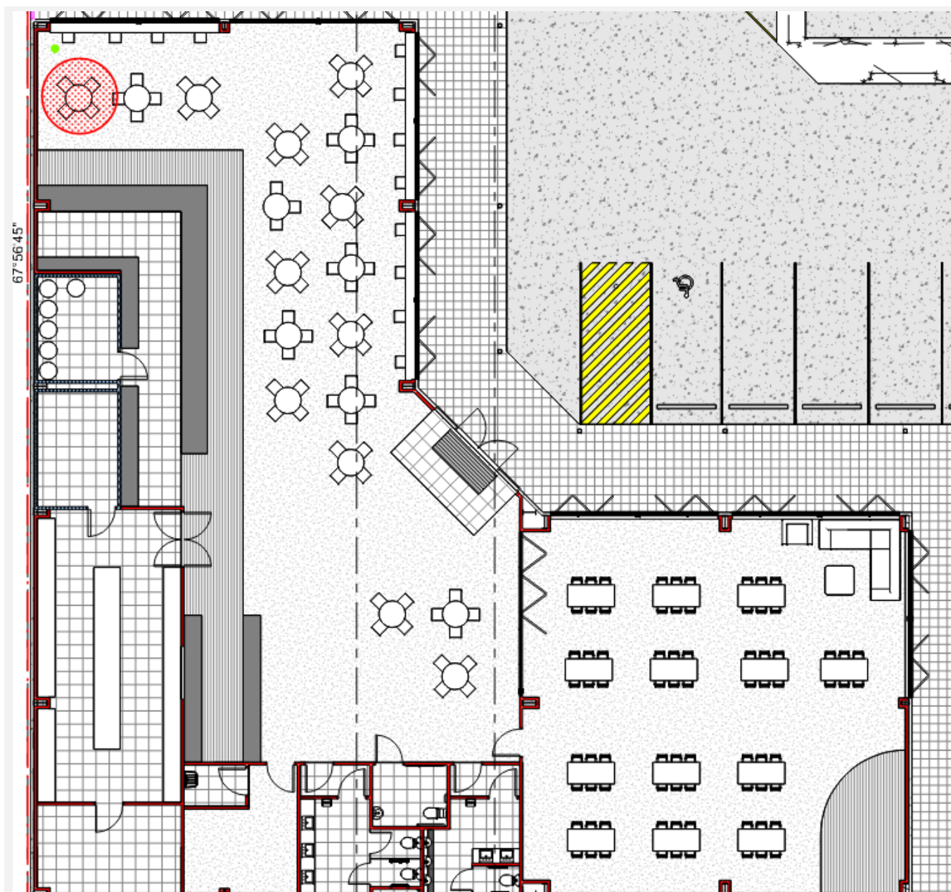
Floor Plan – Table blocking egress path in top corner
